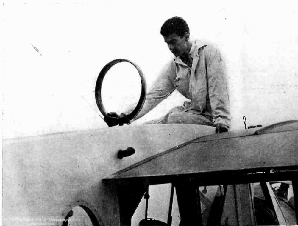
Justus Steele, an employee of the College Park airport, near the Capital City, is seen examining a small round loop mounted on the top of the plane, which may be rotated to bring in the signals from the desired direction
