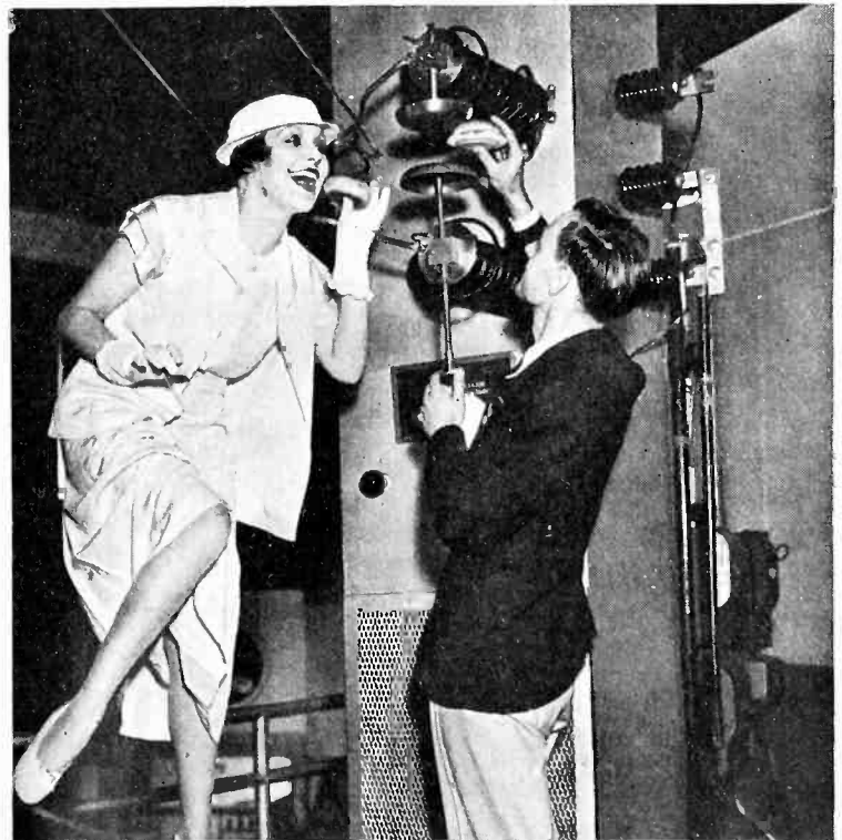
At the Chicago World's Fair, this 20-kw. standing-wave oscillator delivering a 5-meter wave, has been arranged by Westinghouse engineers to toast bun sandwiches by means of the currents induced in the moist bread. This process is similar to that of baking crustless bread "from the inside out" by high-frequency oscillations
