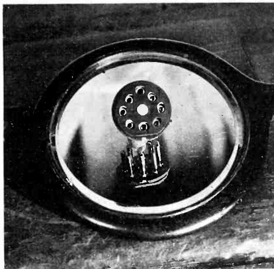
New 8-prong socket for radio tubes under development. The socket is a good example of the use of laminated fiber
