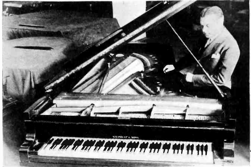
Grand piano used by Berlin Broadcasting stations has its steel strings adjusted to transmit oscillations direct to microphonic device mounted on top
