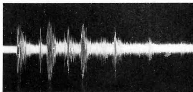
Fig. 6—Oscillograph trace of a multiplicity of echoes often present in auditoriums with large domes or parallel walls
