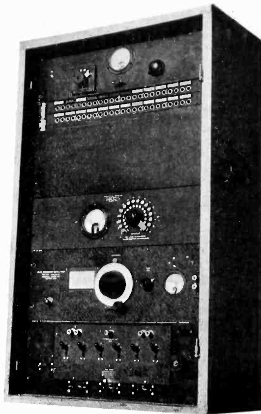
Portable equipment for making gain frequency measurements on studio field units and theater sound equipment
