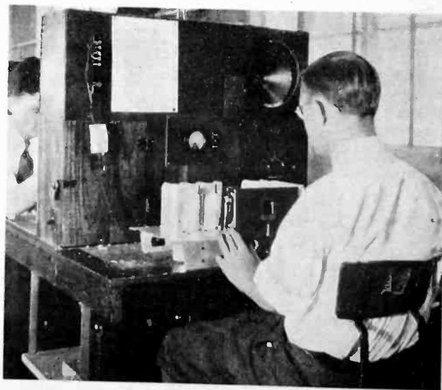
Here radio frequency circuits are adjusted and sensitivity is measured
