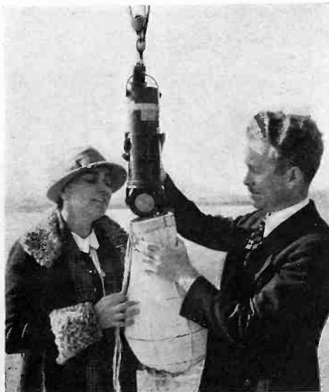
To prevent wind from whistling against the sensitive diaphragm, Paramount's studio engineers devised this microphone jacket for sound picture work
