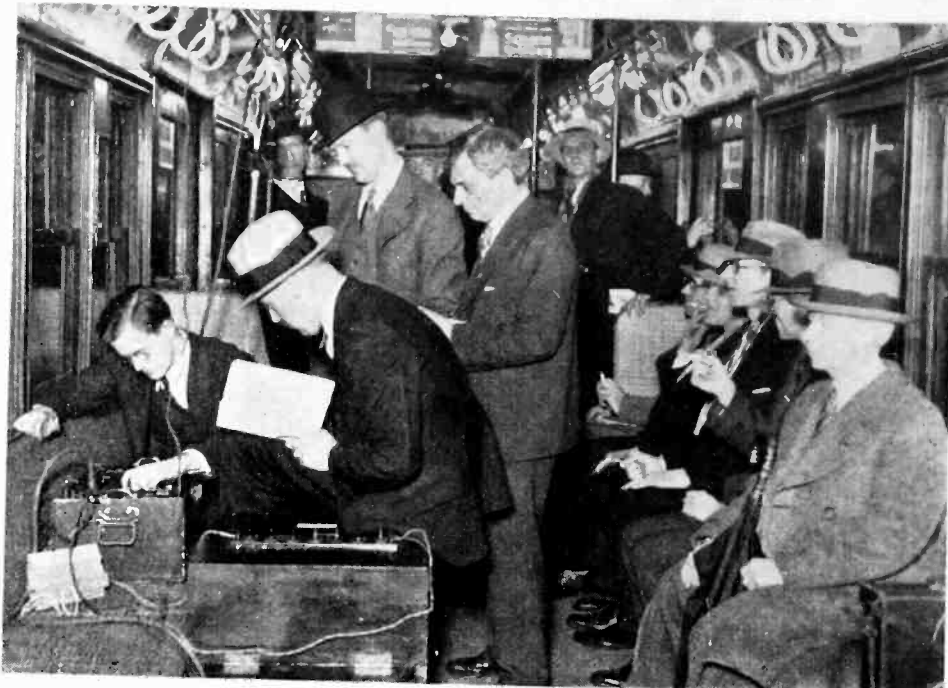
Engineers of Electrical Research Products, Inc., are now making acoustical measurements of noises on New York subways to aid in silencing subway trains
