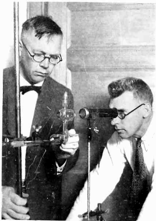
This thermo-couple, used with vacuum-tube amplifiers, will measure one-millionth degree, F. At Mt. Wilson, California, it detects heat rays of stars invisible to naked eye
