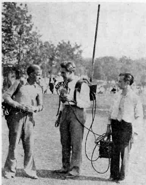
Designed for short wave use this transmitter may be easily carried by two persons in following athletic events
