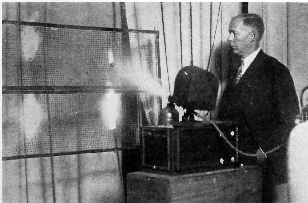
Before the A.I.E.E. at New York, Oct. 24. L. W. Chubb, Westinghouse director of research, demonstrated this "fire scanner." Four flames were lighted on the screen, the scanner was set in motion, and as it came in line with each fire, it stopped, aimed a stream of water, and then, the flame extinguished, went on to the next fire
