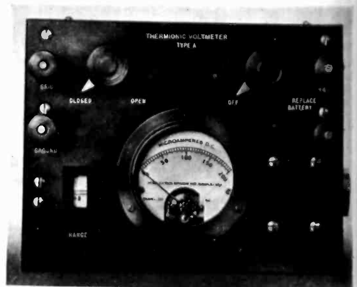
Fig. 6. External view of amplifier-voltmeter
