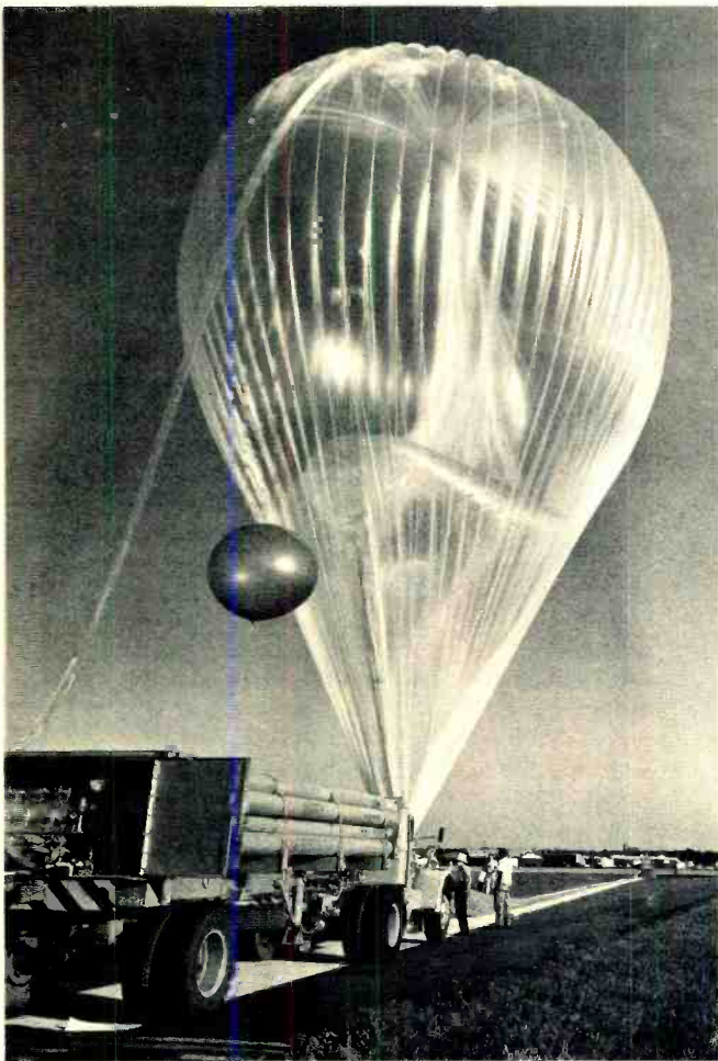
Charging of polyethylene research balloon with 2400-psi truck tanks. Helium is fed through plastic hose on top. Launch spool, mounted in front of truck, restrains balloon during charging.
