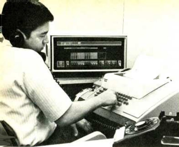
Some models of minicomputers come in "desk-top" versions. This PDP-8/E can be used as an independent terminal for engineering calculations in this configuration. With the modern programming languages available, such as Focal, the computer can be programmed by engineer for use by untrained personnel.
