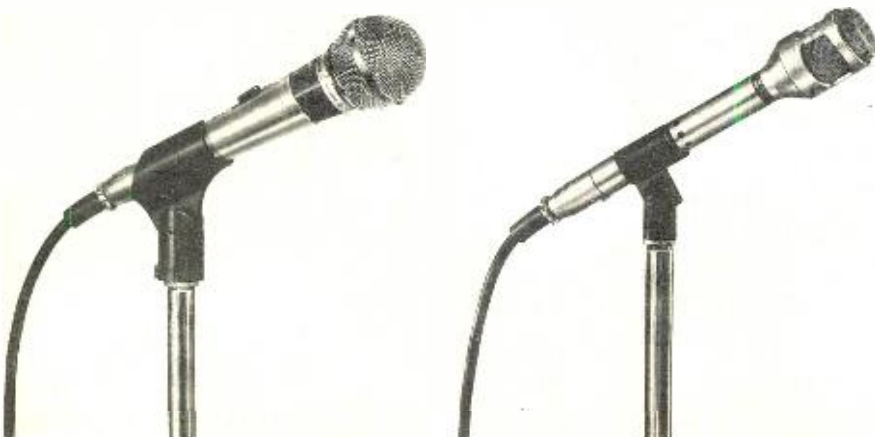
Two unidirectional dynamic microphones suitable for good, portable sound-reinforcement systems. Mike at left has ball-type "pop"-filter and is characterized by proximity effect. Mike at right has integral "pop"-filter and minimized proximity effect as result of holes in handle above mounting bracket.
