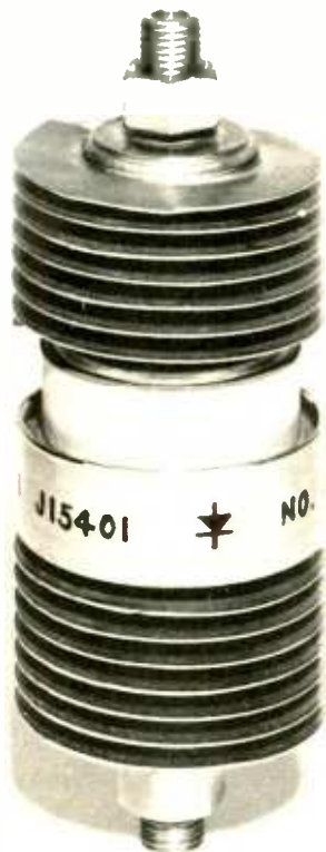
This 250-ampere rectifier uses a combination of a ceramic heat pipe and cooling fins to keep the silicon wafer no more than 10 degrees C warmer than fins. Without the heat pipe, temperature difference would be in excess of 70 degrees C.
