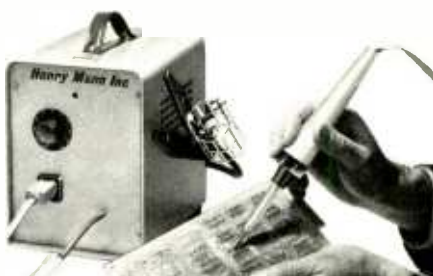
This soldering iron is operated from solid-state variable supply.
