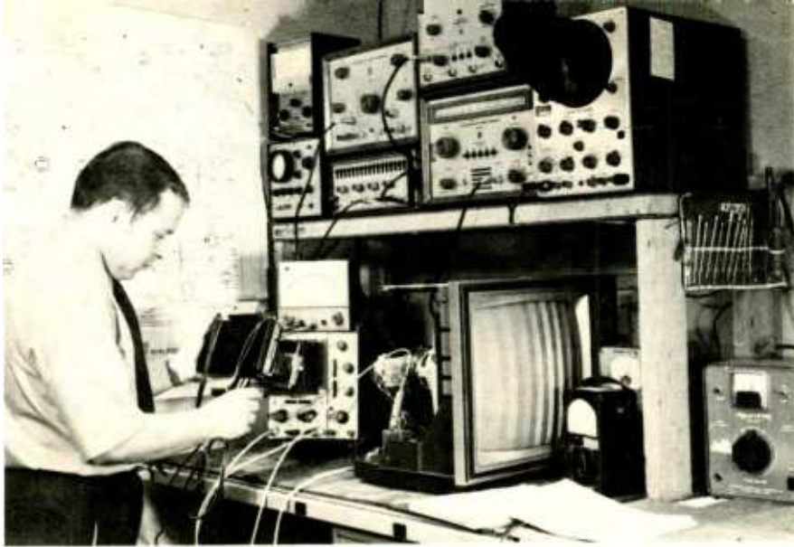
◀ The technician uses a whole battery of TV test equipment for making the waveform photos that are then used in TV service manuals.
