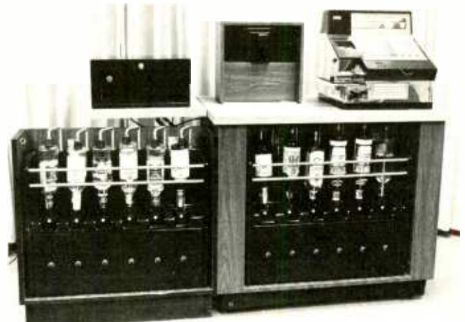
Fig. 1. The automatic bartender is composed of five units: (1) the control register, (2) the logic unit, (3) the liquor-bottle racks, (4) drink-dispensing head, and (5) compressor.
