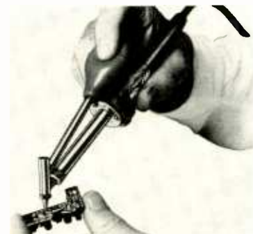
Combination desoldering-resoldering iron made by Endeco.
