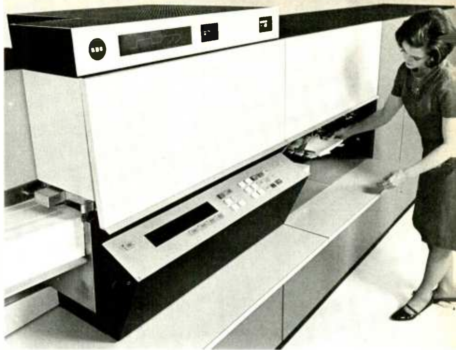
The IBM 1288 OCR system, besides reading handwritten numbers, five handwritten alphabetic characters, and all the standard computer alphanumeric characters printed by machine like its predecessor, the IBM 1287, can also read Gothic type. The Model 1288, introduced in early 1970, rents for $4755 per month, costs $223,390, must be used in conjunction with a 360 computer.
