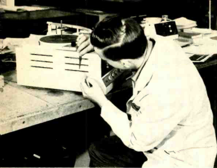
Investigating possible shock hazards in a record player, the technician is measuring the size of the ventilating openings to see if additional probing tests are needed to check any live parts that may be accessible inside the enclosure used.
