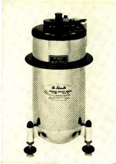
Fig. 7. Worden gravity meter. Instrument is used to survey craters when magnetometer approach is too complex.
