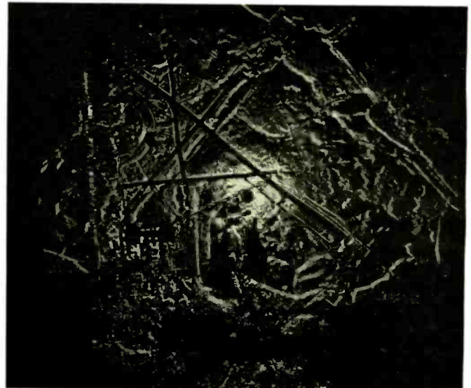
High-resolution ASDE radar display. Note the clear demarcation of the buildings, runways, and ramps of the airport.
