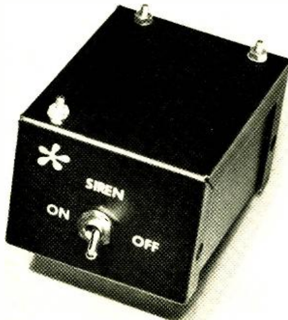
Power siren with automatic cycling showing siren "On-Off" switch.
