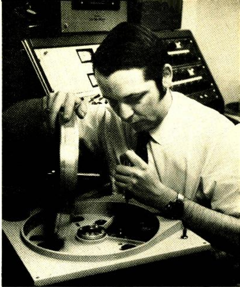
Routine maintenance of station equipment is required. Here the author is tightening motor mount in the studio turntable.
