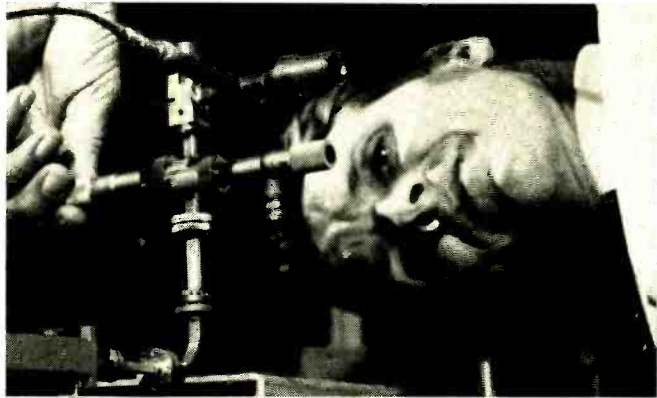
Millimeter-wave repeaters will be required every 20 miles. The components for such repeaters are now being lab-tested.
