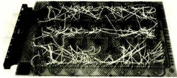
This one-piece, economy-type 40-terminal, card-edge connector is employed in a new automatic writing machine.
