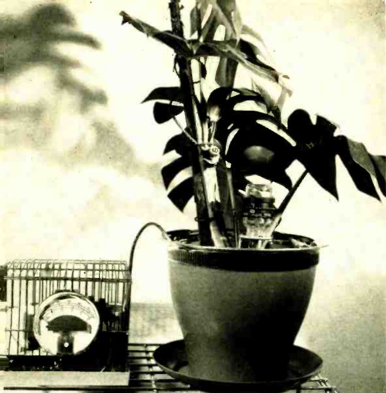
Fig. 8. Indoor arrangement for testing Backster Effect. The d.c. amplifier is at left, connected by shielded line to the leaf and set-up potentiometer. Nutrient feeder is in the pot.
