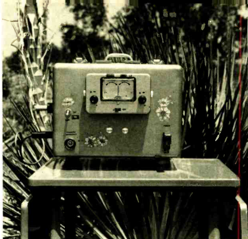
Fig. 11. The d.c. galvanometer and packaged electronics devised for testing the emotion-like response of yucca plants outdoors. The plant shown in the lead photo indicates size.
