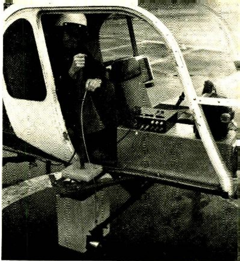
John Wear of U.S. Forest Service's Pacific Southwest Forest and Range Experiment Station prepares equipment that will be used to take temperature of trees. The housing attached to the underframe of the helicopter contains heat sensor, TV camera.
