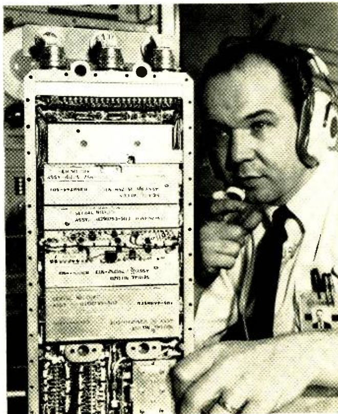
An opened extra vehicular communications system radio similar to the ones used by our astronauts is being tested here.
