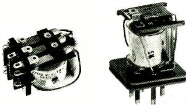
Fig. 3. A pair of relays that are designed for a.c. operation.
