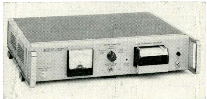
Fig. 5. Automatic phase-tracking 60-kHz receiver makes continuous strip-chart recording which compares reception of NBS station WWVB with a local oscillator. Comparisons are easily reliable beyond parts in 10^9 at almost any reception point throughout the U.S. Tracking, if carried on daily and averaged over several days, are capable of making comparisons within parts in 10^{11} accuracies.
