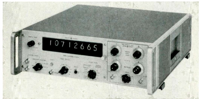
Fig. 4. A highly accurate electronic counter with an 8-digit display and time-base stability better than 3 parts in 10^9 per day.
