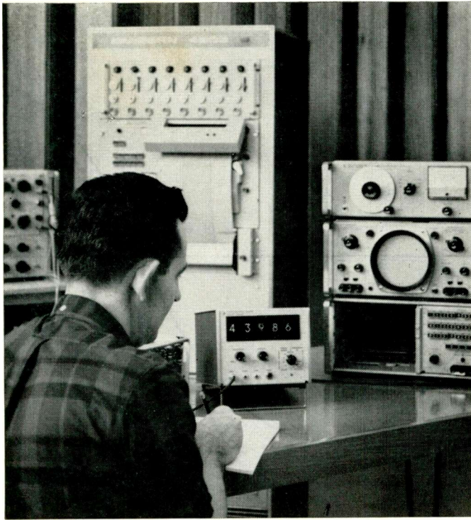
Fig. 1. A counter of medium stability with 5-digit readout is shown here. Aging rate is specified as parts in 10^6 per week. Crystal used is of high quality but is not enclosed in an oven.
