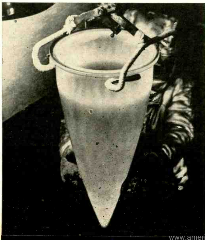
Fig. 2. High-temperature, high-strength glass-ceramics are used as combination nose cone/radome in many guided missiles.
