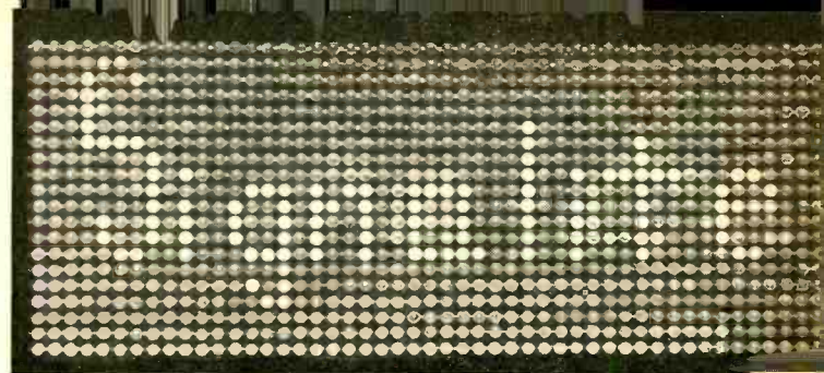
The message to be displayed is written with a small flashlight "pencil" on a glass plate. The display itself, shown here, consists of a bank of 1000 special neon glow lamps.
