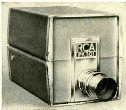
RCA Model PK-301. Fully transistorized, uses new 1" electrostatic focus vidicon and provides 700-line resolution. Aperture and gamma correction. Light compensation range: 2000 to 1. Bandwidth: 8 mc.
