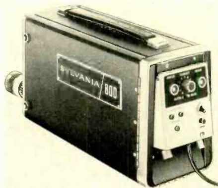
Sylvania Model 800. Rear panel is removable permitting use of extension cables for remote locations. Resolution: 800 lines. Bandwidth: 10 mc. A.l.c.: 4000 to 1. Voltage regulated. Transistor circuitry.
