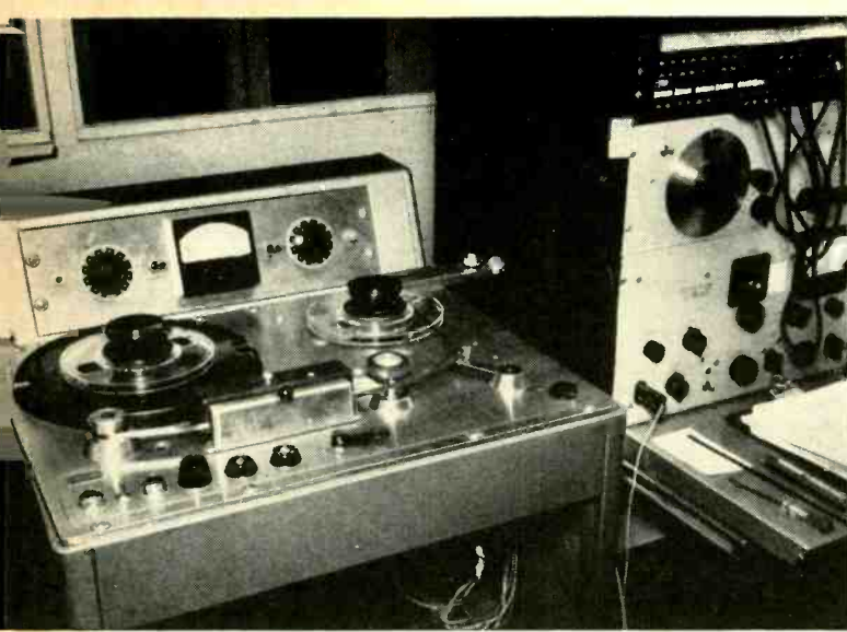
Quarter-inch recorder instrumented for secondary electromagnetic measurements in accordance with Navy specification WT-0070.
