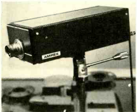
Ampex Model 322 closed-circuit camera. Resolution: 600 lines. Bandwidth: 7.5 megacycles. A.I.c. 2000 to 1. All transistor.
