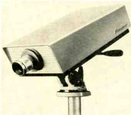
North American Philips, Norelco Model EL8000/11 closed-circuit television camera. Unit is compact, lightweight. Resolution: 450 lines. Bandwidth: 5.5 mc. A.l.c.: 15 to 1. Circuit is transistorized.
