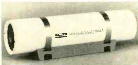
Cohu/KinTel Model 2000. In environmental housing for temperature, explosion, pressure, and humidity extremes. Narrow diameter for insertion into pipes. Resolution: 700+ lines. Bandwidth: 10 mc. A.I.c.: 4000 to 1. Voltage regulated, transistorized.
