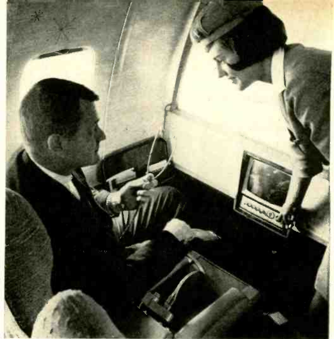
Stewardess instructs a passenger in use of Astrovision. At passenger's right elbow is earphone jack and volume control.
