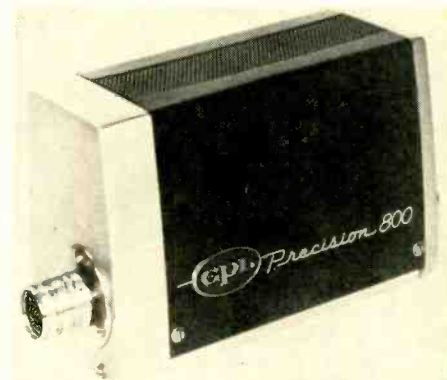
General Precision Labs Model GPL800. Camera and control chassis are separate for remote control. Resolution: 800+ lines. Bandwidth: 12 megacycles. A.l.c.: 6000 to 1. The circuit employed is a hybrid.
