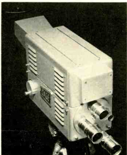
Dage Model 320B. Camera and control chassis are in separate housings for remote control. Resolution: 700 lines. Bandwidth: 8 mc. A.I.c.: 4000 to 1. The circuit employs tubes. Camera is voltage regulated.
