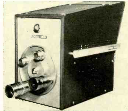
Blonder-Tongue Model EV-1 viewfinder camera designed especially for educational TV. Resolution: 800 lines. Bandwidth: 10 mc. A.I.c.: 4000 to 1. The electronic circuit employed is transistorized and regulated.
