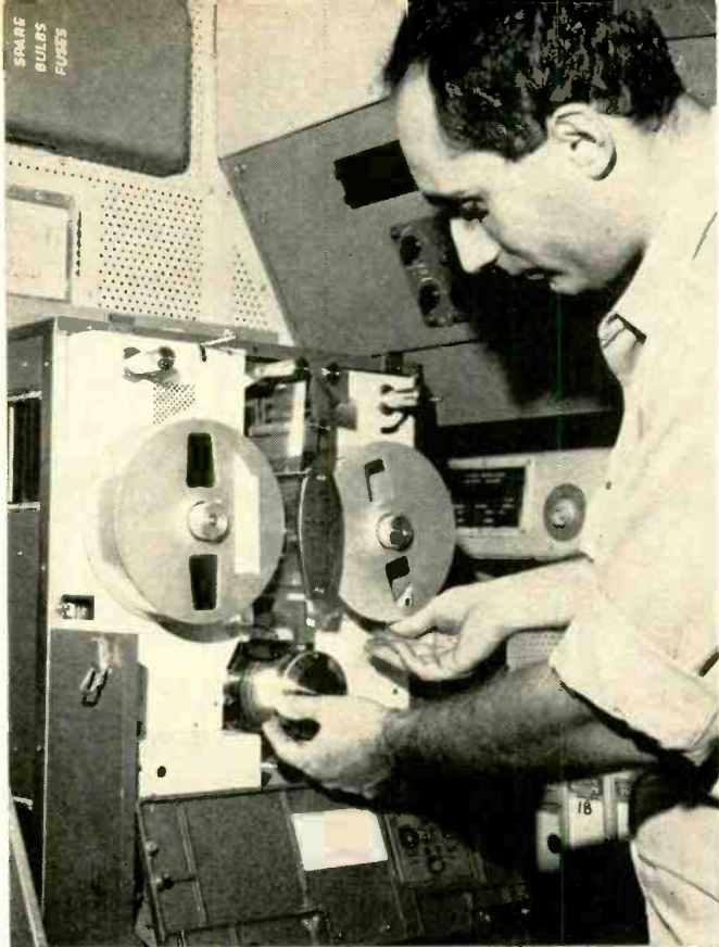
Airlines technician is shown changing tapes on the plane's video tape recorder. About 120 minutes of entertainment are provided on a single reel of specially prepared tape.
