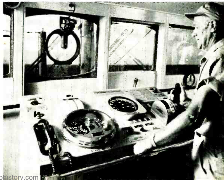
The new look in ship's bridges. Using electronic circuits, the ship's throttle can now be controlled from the bridge.
