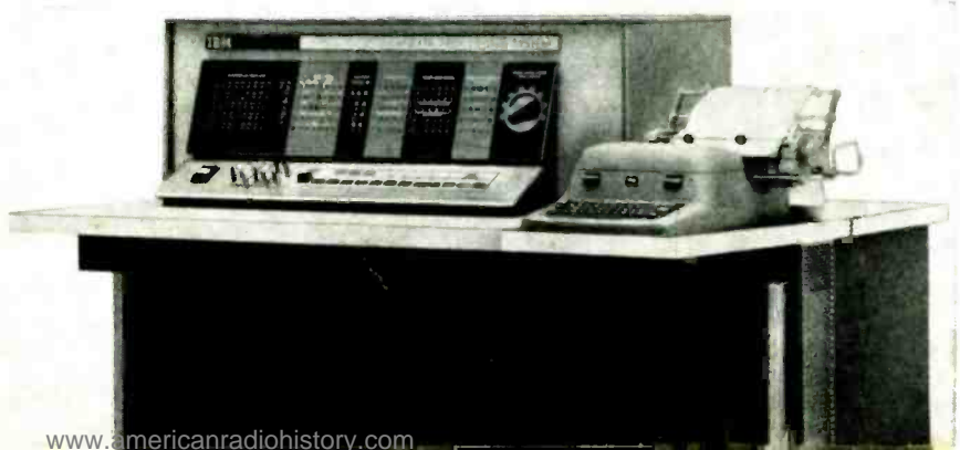
Fig. 3. Perforated tape is used to store programs and data for computers. Positions of holes represent digits, letters, punctuation. This data-processing system employs an input-output typewriter shown at the right of console, perforated tape punch and reader, left.
