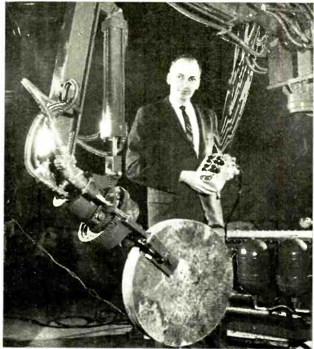
Underwater Mechanical Arm. (Above) This rugged underwater mechanical arm designed to recover objects from the ocean's depths is shown being tested prior to delivery to the Navy. The arm consists of a 10-foot-long hydraulic structure whose operation is electronically controlled by means of an ACF Industries control system. The arm is now attached to the underside of the bathyscaphe Trieste, and can be used to pick up from the ocean floor objects weighing in excess of 500 lbs.
