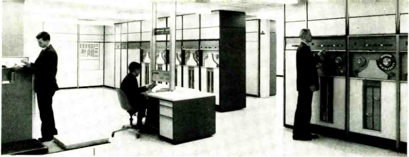
Another typical computer system. Operator's console is at center, punched-card machine at left, and tape machines at right. The "wall" in left background is central processor used with system.
