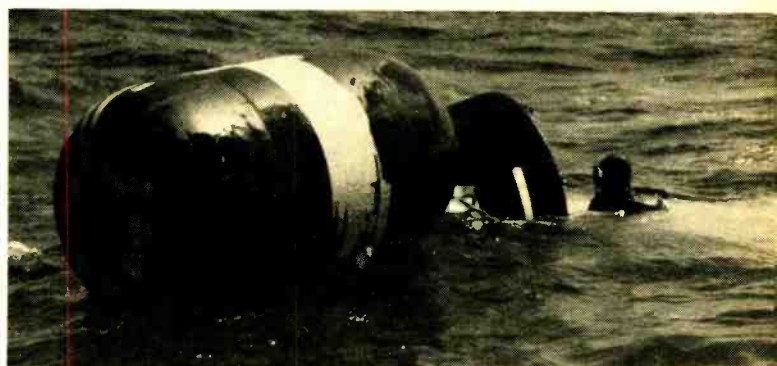
An inflated bag is secured to an Atlas nose cone after it has landed in the ocean. This particular nose cone flew 5000 miles.
