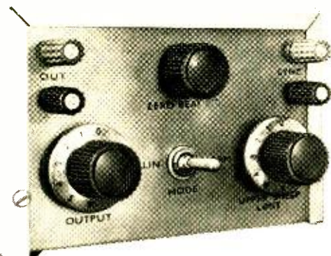
Front-panel view of the author's compact a.f. sweep generator.
