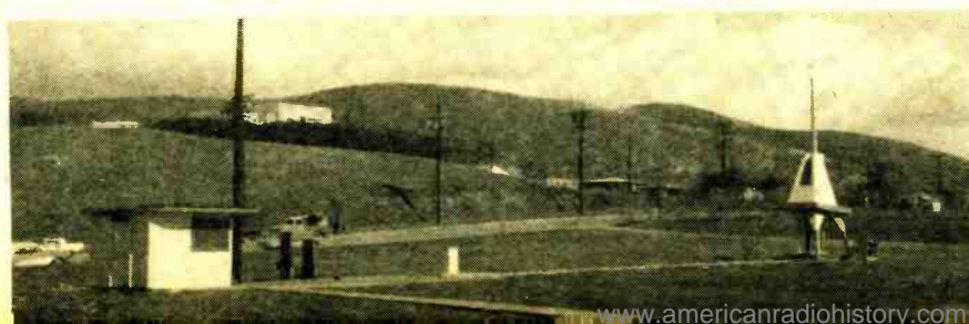
Fig. 3. In the actual test range, the u.h.f. converter under test is connected to the antenna on the right. The small house on the left contains the u.h.f. receiver used for calibration.
