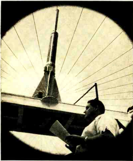
Long-Distance Communications Antenna. (Left) A new antenna that will facilitate long-distance communications with the U.S. Air Force's missile-tracking ships has been designed by ITT Federal Labs. The antenna uses a remotely tunable helical loading coil plus top-hat loading. The fan of wires is a ground plane. Tuning range is 2 to 30 mc. with power-handling capability of over 10 kw. peak envelope power. . . . Laser Tracking System. (Below) An experimental optical-frequency tracking system that tracks laser-illuminated targets is now being tested by Westinghouse. The transmitter, at left, and receiver, at center, are being manually aimed at a target. The two meters that are shown at the lower right corner of the photograph indicate the azimuth and elevation errors.
