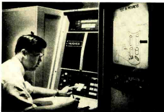
(Left) "D-PAT" uses a digital computer with a test program stored on a magnetic memory drum. After going through an extensive automatic testing procedure, the unit flashes repair instructions on a viewing screen, displaying a picture of the malfunctioning assembly with a bright red arrow pointing to the part causing the trouble. (Right) A coded Mylar tape is being inserted into "TAPAT" (Tape Programmed Automatic Tester). The unit cuts the time and cost of inspection of printed circuit cards and allows the tests that are made by the system to be monitored readily by means of non-technical personnel.
