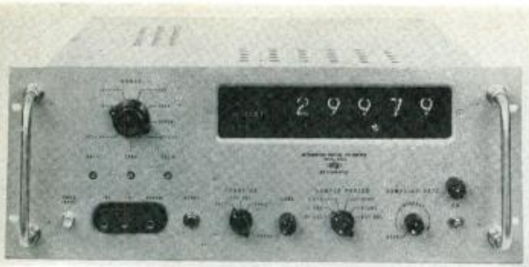
Fig. 2. Dymec Model 2401A is capable of five-place accuracy.
