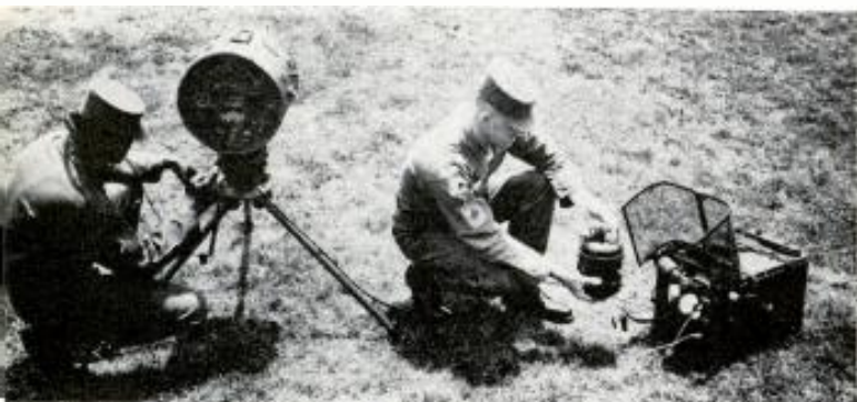
Soldier at right is shown loading a new fuel supply. Metal hydrides in the tank generate hydrogen to power the cell. This unit supplies enough power for the portable radar set at left.
