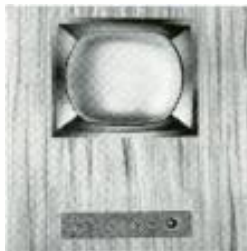
Custom wall installation of "DeLuxe" Color Chassis with horizontal controls separated from chassis.
