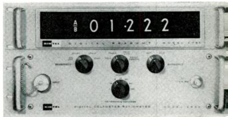
Fig. 6. A typical ratiometer. It indicates the ratio of the test voltage A to internally generated reference voltage B.
