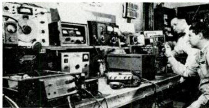
Photographs showing a pair of typical service-bench setups for handling mobile two-way radio equipment.
