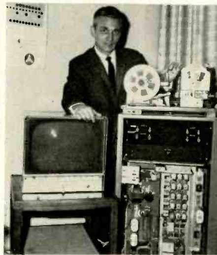
Tape-programmed equipment at right determines who of up to 10,000 subscribers have their company-supplied speaker turned on.
