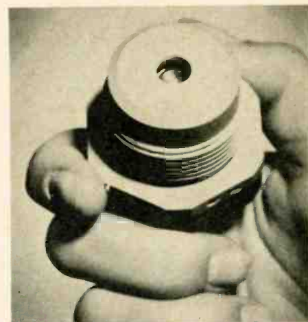
Fig. 6. Polarographic oxygen sensor is rugged; used in space and oceanographic work.
