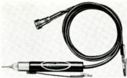
Fig. 2. With a detector probe, your meter checks signal up to v.h.f. frequencies.
