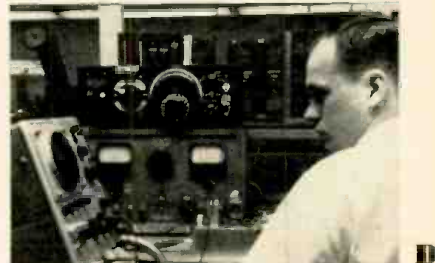
C. James Ortloff breadboards a section of circuitry for new test equipment. Visual inspection is of little use in making computers and generalized types of test equipment require too much time to use. Instead specialized and sophisticated test gear is commonly employed.
