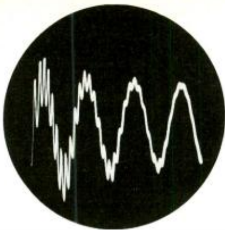
Fig. 4. Damped waveform of Fig. 3 with the scope's frequency controls re-set.
