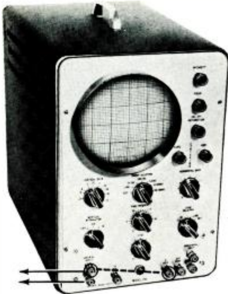
Fig. 11. Binding post for blanking output (right) is temporarily connected to vertical input (broken line), with latter connected (arrows) to external circuit.
