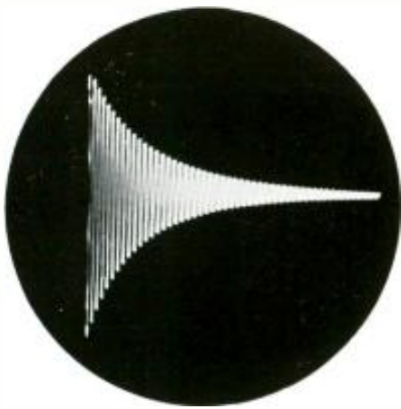
Fig. 1. Damped oscillation in flyback transformer with h.v. rectifier removed.
