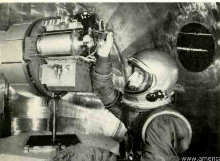
▲ This Plasmadyne Corp. arc-jet engine weighs 12 pounds complete with fuel, delivers a fraction of a pound of thrust, and is not much bigger than a football. It may be used to nudge space satellites into exact orbit and for other precise space functions.
