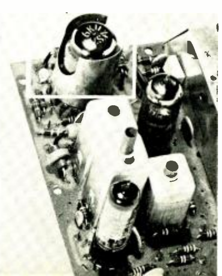
Fig. 2. In space taken by conventional tube, a 6K11 (in box) serves 3 stages.
