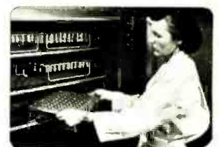
Gun mounts are dried for one hour at 150°C (302°F.). Then, super-dry and super-clean, they are taken out for final processing in our dust-free "White Room".
