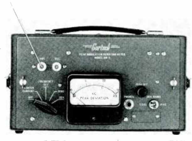
Fig. 5. The Gertsch Peak Modulation Deviation Meter, Model DM-3, is typical of deviation monitors used to set audio clip-pers. This setting keeps modulation within permissible limits.
