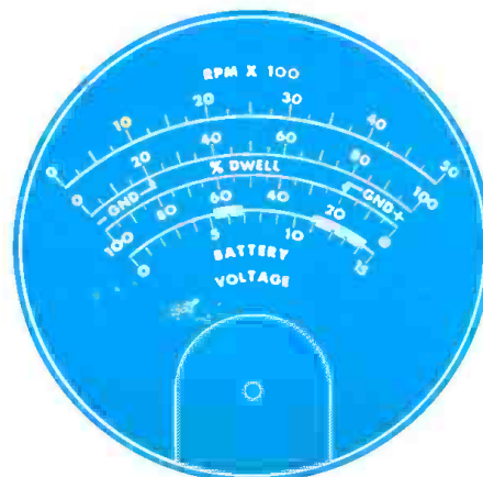
Fig. 2. The new meter scales used by the authors. The top scale indicates engine speed, the next two scales indicate dwell per-cent for cars with either a negative or a positive ground system, and the bottom scale indicates the voltage of the battery.
