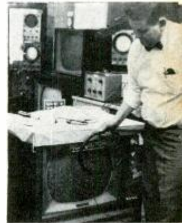
Fig. 1. A degaussing coil is being used to demagnetize a color picture tube.
