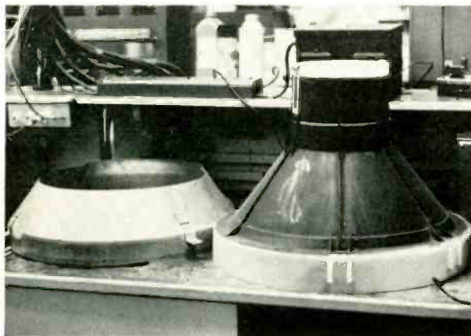
Fig. 2. Compare new CRT shield (left) with old shield (right).
