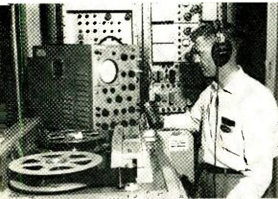
Operator of a Videotape TV recorder at the White Sands Missile Range's Signal Missile Support Agency, New Mexico, is shown here checking out the performance of the system. The tape recorder records radar signals picked up from a missile in flight.
