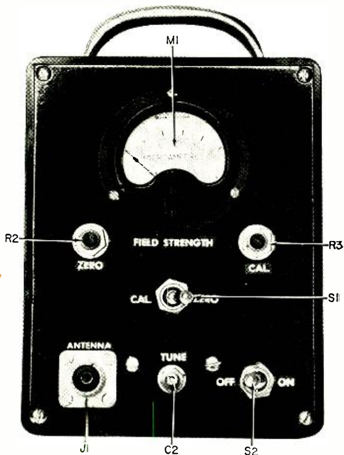
Front-panel view of the author's home-built field-strength unit.
