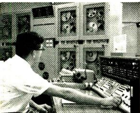
Control console of a large computer that employs a number of magnetic tape recorders. This electronic system handles 33,000 accounts an hour, requiring only 32 \mu sec. to perform each step of sorting, reading, and computing from face of bank checks.
