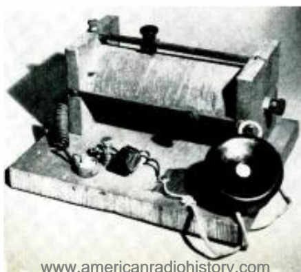
Fig. 1. Ham construction in pioneer days was crude with few commercial parts. This receiver, with "two-slide tuner," used a corundum crystal detector, home-made fixed capacitor, and single 75-ohm "watchcase" telephone receiver. A hand-sawed breadboard base mounted all the components.
