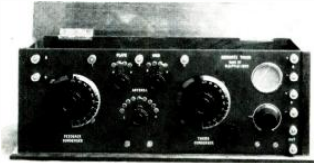
Fig. 2. This receiver, built in 1922 by Author Pyle, employed a wooden cabinet with a hard-rubber front panel. Machine engraving had come into vogue and enhanced the set's appearance.
