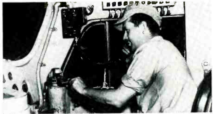
Radiotelephone handset being used by engineer of diesel-electric freight locomotive on the B & O's radio traffic control system.
