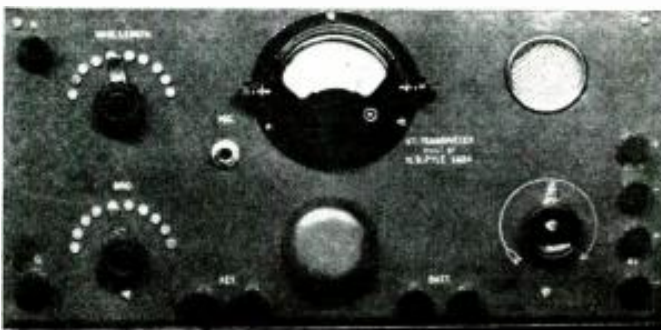
Fig. 4. Ham phone transmitter built by author in 1924. This 5-watt rig used "loop modulation," produced by wrapping single turn around tuning coil and connecting it to microphone through a mike battery.
