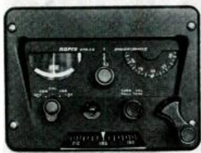
VOR receiver. "Left-Right" meter with "To-From" indication, is at left. The course-selector dial is at the bottom.
