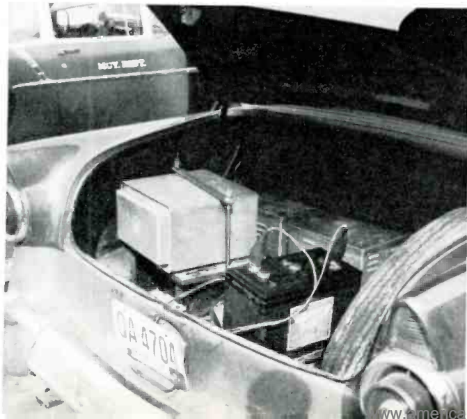
Fig. 3. Radar set installed in trunk compartment of car.
