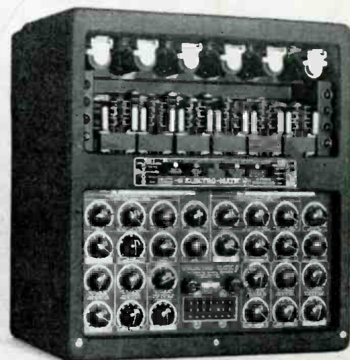
Fig. 11. Front panel of the versatile traffic controller described in text.
