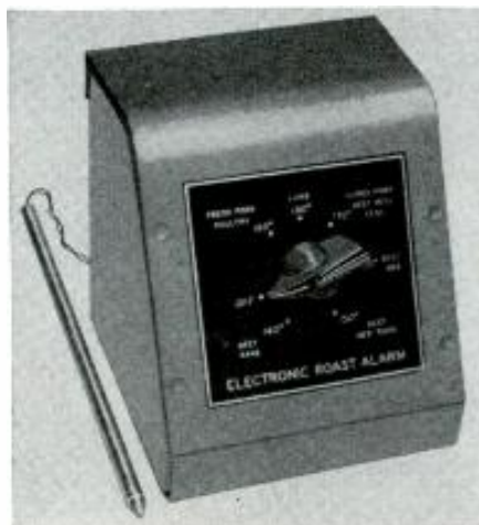
Fig. 2. Roast alarm control box with the temperature scale on the front panel.
