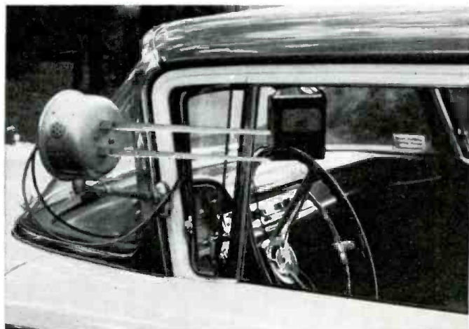
Fig. 8. Installation of r.f. unit of X-band (10,525 mc.) radar.
