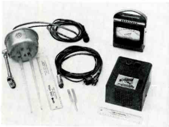
Fig. 9. Complete X-band radar. Note dielectric antenna rods.
