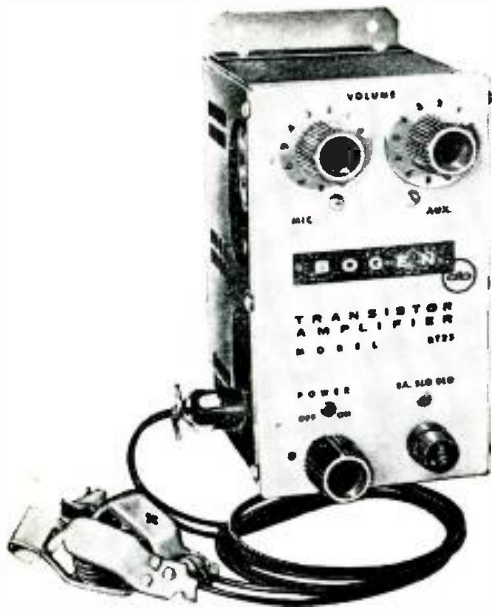
Close-up view of the 25-watt mobile transistorized amplifier designed for p.a. work.
