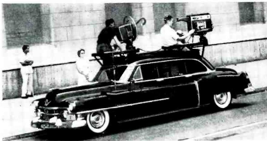
NBC Cadillac used microwave relay atop the car for good on-the-move coverage.
