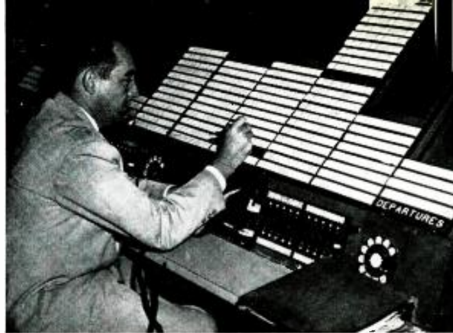
A New York area traffic controller keeping track of aircraft movements by noting flight location on flight progress strip.
