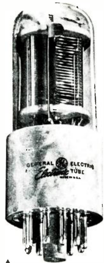
Fig. 1. The General Electric 931-A photomultiplier. The grille structure visible in photo allows light to pass to cathode and provides electrostatic control field.
