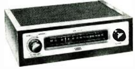
This AM tuner is completely a.c. operated, employing 6 tubes and a special DM70 type tuning eye. Output is a plate-follower type, having an impedance of 8000 ohms.
