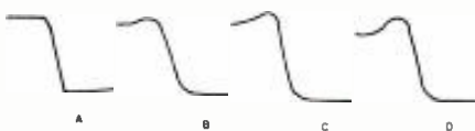
Fig. 7. Trailing edge of square wave (A) before effect of compensation and after alteration (B, C, and D) by various positions of circuit in Fig. 6.
