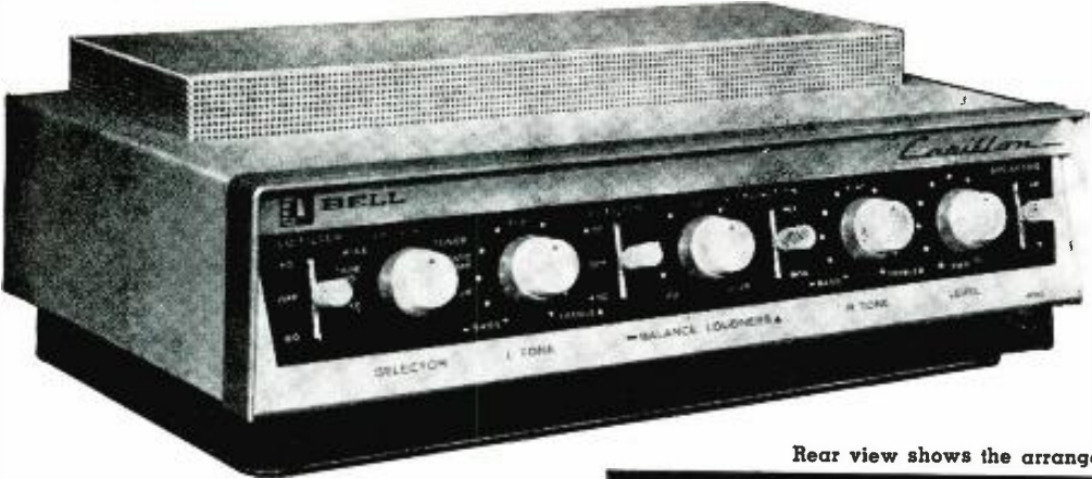
Over-all view of the "Carillon"—a new dual 30-watt integrated stereo amplifier.
