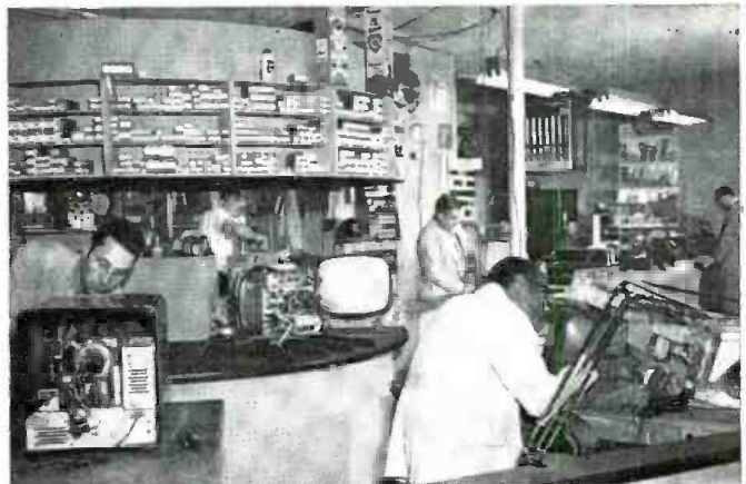
Fig. 4. Overhead rotary shuttle carries stock of tubes, lower shuttle carries sets to advanced-service benches.
