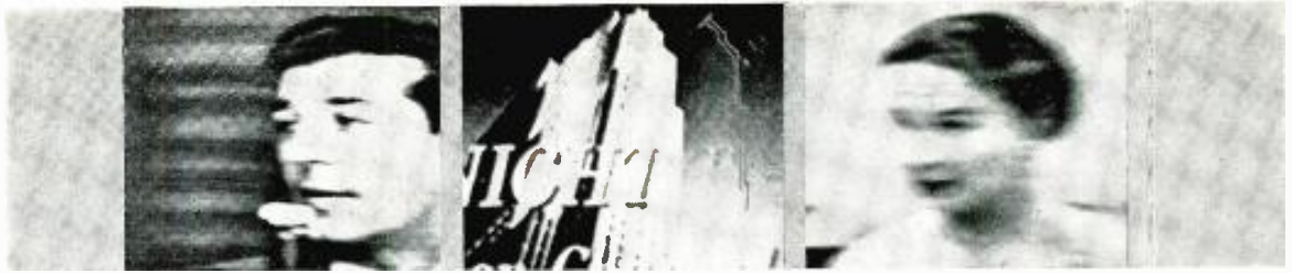
Fig. 1 (left). "Weaving" pattern superimposed on the picture. Fig. 2 (center). Definite, displaced ghost. Fig. 3 (right). Poor resolution may be caused by misalignment, antenna-system mismatch, or a "close" ghost.
