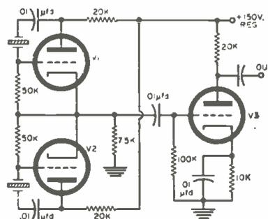
Fig. 1. A simple twin oscillator. Output capacitor may be .001  $\mu$ fd.
