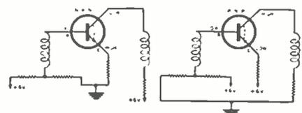
Fig. 8. Emitter-to-collector leakage.
