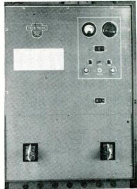
Fig. 8. Photo above shows the front panel of a 7.5-kw. induction heating generator. Note simplicity of the controls required.
