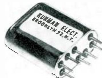
ture range is from -65 degrees C to +125 degrees C. Sensitivity is 200-250 milliwatts. The new model is offered in three different header combinations. The relay will withstand shock tests of 50 G's; vibration frequency of 20 to 2000 cps at 20 G's. Coil resistance is up to 10,000 ohms maximum and contact resistance is .020 ohm maximum.
