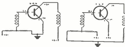
Fig. 7. Open lead in transistor base.
