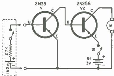
Fig. 2. Diagram of a less sensitive motor control circuit. An input control signal of ½ milliamperes will operate the motor. The several components within the dashed lines may be used for testing the circuit. These will provide an input control current of ½ ma. A penlite cell may be employed.
