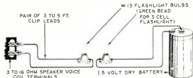
Fig. 1. Simple lamp comparator as is discussed in the text.
