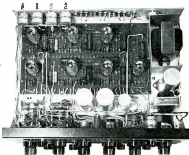
Top view shows printed circuit assembly and general arrangement of parts.
