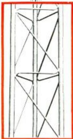
**No. 25** The ROHN No. 25 tower is one of the finest ever designed . . . a full 33% stronger and more durable than "similar sized" towers. This is achieved by amazing zig-zag cross bracing design combined with highest grade steel and heavy-duty steel side-rail tubing. This superior strength means that this tower can ordinarily be installed self-supporting to 50 feet or guyed to 200! It is truly the finest tower of its kind for home television reception.
