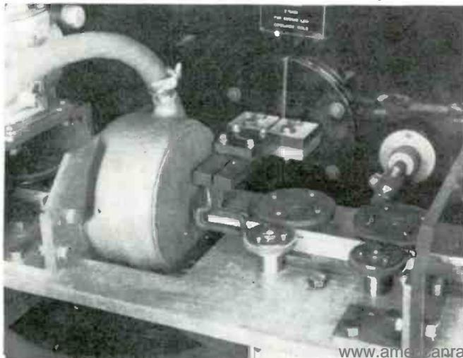
Fig. 4. Moving coil fixtures for heating, bending door handles.
