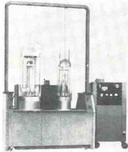
In bending, for example, only the area of the bend itself need be heated and since induction heating does this so quickly, the rest of the work piece will remain rigid and retain its shape. Fig. 4 shows a moving coil fixture in which an aluminum door handle is heated to 900° F and bent at right angles in 3 seconds, the entire operation being completely automatic, accurately controlled, and without forming scales, discoloring, or distorting.
