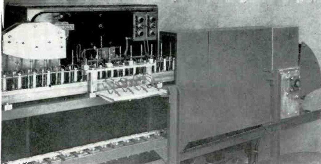
◀ Fig. 1. A conveyor carries beaters for home mixing machines through this induction heating unit which brazes the beater blades to the main stems automatically.
