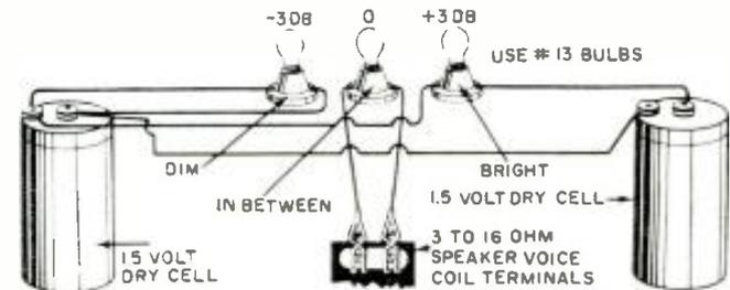
Fig. 2. A somewhat more accurate lamp output meter is shown.
