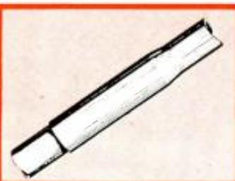
**Tubing**—Just what you want: 6" expanded end with 1/2" taper to form a solid locking joint! High carbon steel. Available 5, 10 foot lengths, 1 1/4", 1 1/2" diameter, 16 and 18 gauge.
