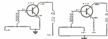
Fig. 4. Open condition in the emitter.
