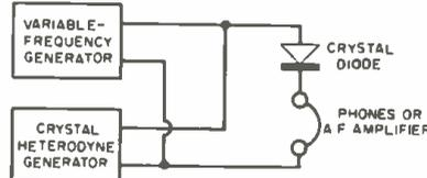
or any other comparable combination of available crystals. With the latter, no fundamental (or other strong beat) would be close to the desired frequency. When use of a "close" combination is unavoidable, a careful search should be made to find *all* output frequencies. The desired one may be identified by its location relative to the others in their fixed sequence.
