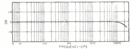
Fig. 4. Frequency response of amplifier.
