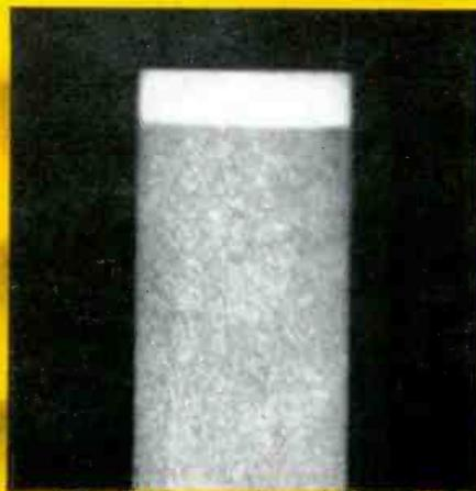
Inherent physical superiority of Sylvania's exclusive Sarong cathode, right, over a conventional cathode, left, is evident in this photomicrograph comparison. The texture,
