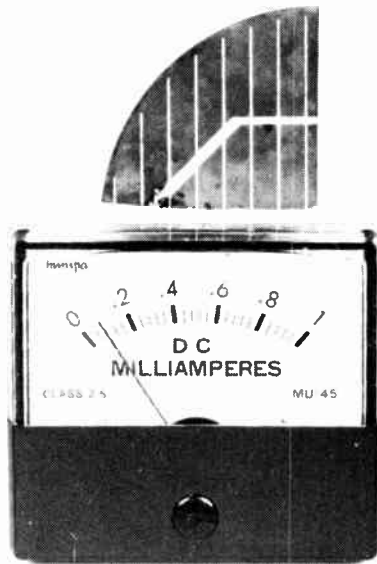
Front view of the sun intensity meter we made as an experiment. The cell we used is a Sensor Tech, C202, quarter of a C200.
