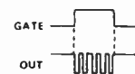
Figure 11. A variation on the circuit in Figure 10 allowing gated operation of the multivibrator.
