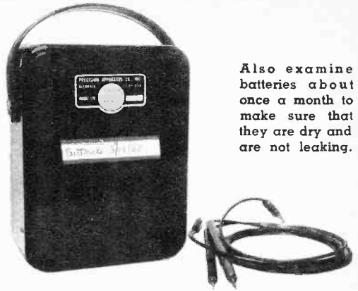
When did you install batteries in that meter? A label on the back of the meter will remind you.
