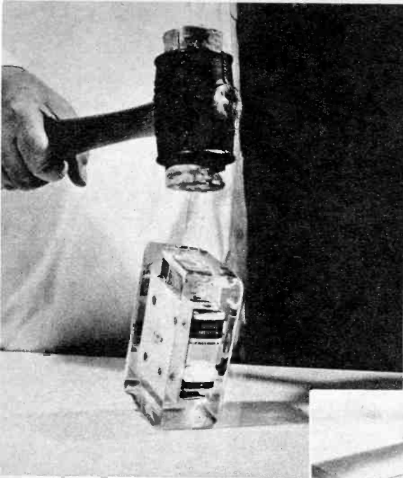
Photo shows the cushioning protection that is afforded by General Electric's clear potting compound, LTV602. The test is not recommended if the subassembly includes delicate electronic parts.
