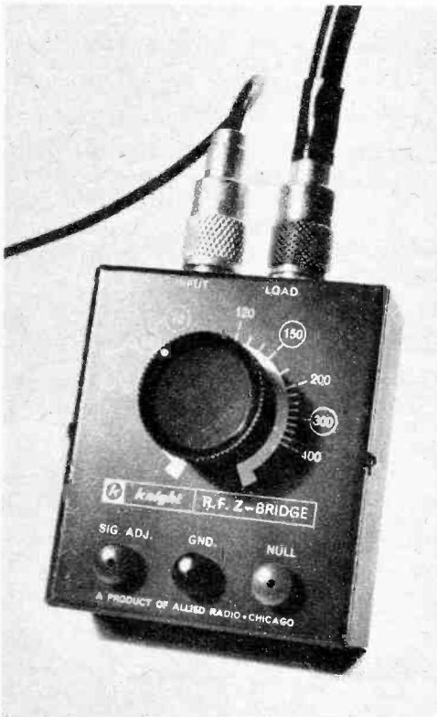
Impedance bridge is useful device for checking elements of antenna system. It has one control.
