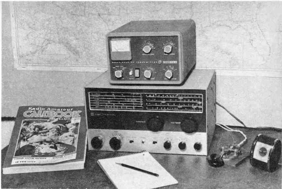
Excellent basic station setup for the beginner; Knight-Kit R-55 receiver with Eico 723 transmitter on top. Both are simple kit projects. The call book, key, and clock are necessary accessories in the ham shack.
