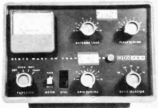
To save time when retuning a transmitter, mark settings of frequently used frequencies on tapes.
