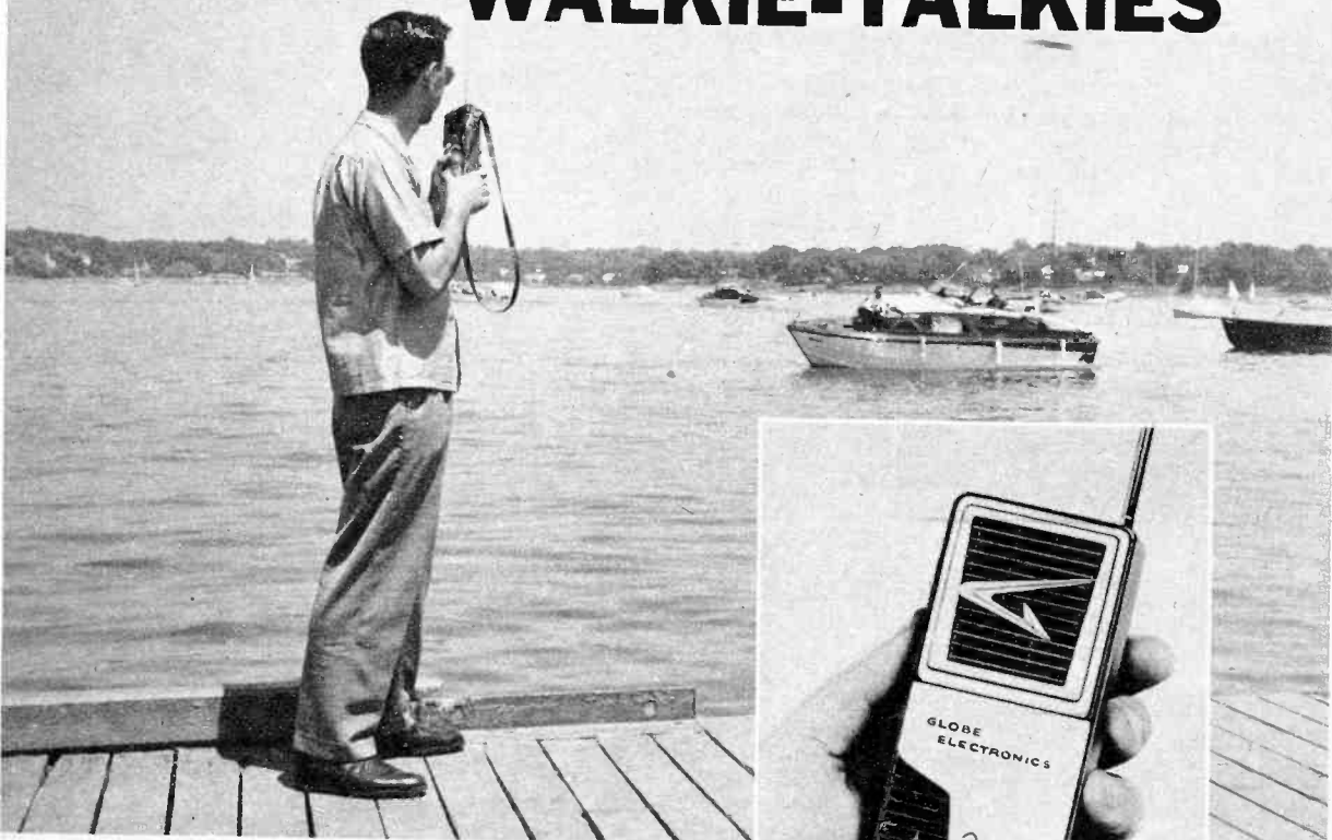
Above: Instant push-to-talk communication over water is possible with hand-held, low-power transceivers. The Globe Electronics Pocketphone is representative of units.
