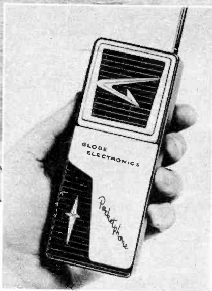
Above: Instant push-to-talk communication over water is possible with hand-held, low-power transceivers. The Globe Electronics Pocketphone is representative of units.
