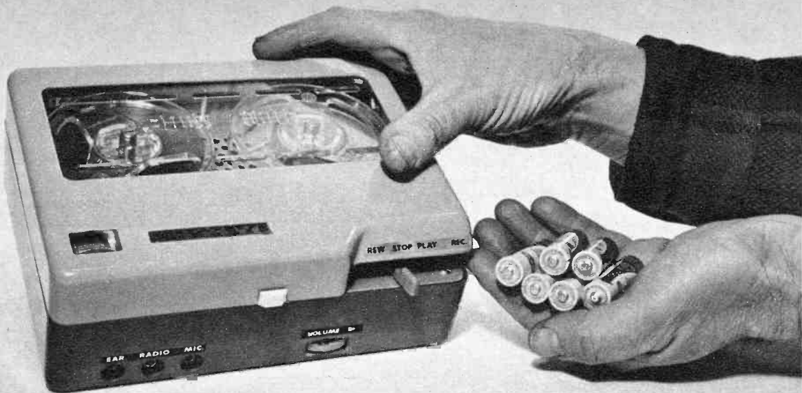
Small size and low power requirements of transistors make possible compact, self-contained instruments. Here is a representative tape recorder (Lafayette RK-120); it is powered by just six standard penlight cells.
