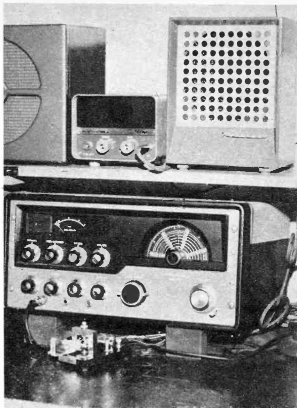
Hallicrafters Model HA-1 electronic keyer occupies little space on shelf between loudspeakers. Poucel "Elkey" is on table in front of receiver.
