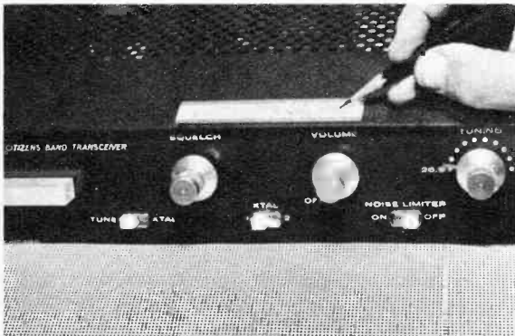
What channel is that CB transmitter operating on? After installing xtal, mark frequency on label.
