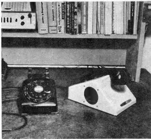
This view shows the sound reflecting surface of the amplifier case in which the mike end of the handset should face. Position is reversed here.
