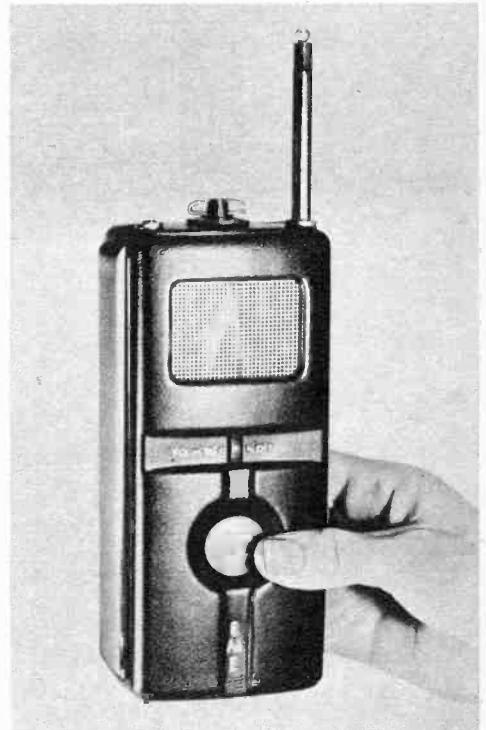
RME 4304 transceiver control switch is at bottom, speaker at top. An earphone jack is also provided.
