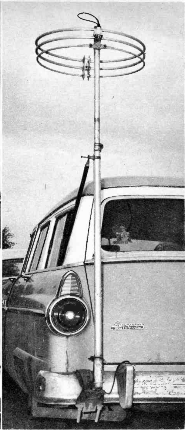
These are two popular types of mobile antennas for 2-meter operation. The left is a straight coaxial whip, which has advantages of slimness and minimum wind whip. At the right is a "halo," which is heavier and larger but operates like a beam in that it gives additional gain over a straight whip antenna.
