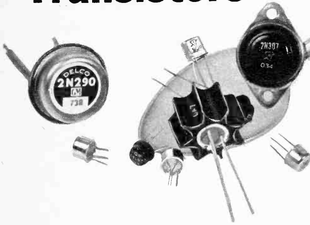
Many sizes and shapes, but all small. Collection of typical transistors in spoon for size comparison. Larger ones are used in high-power applications.
