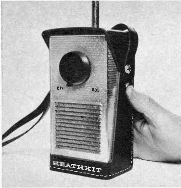
Volume control and push-to-talk switch are only controls on Heath GW-30. Antenna is collapsible.
