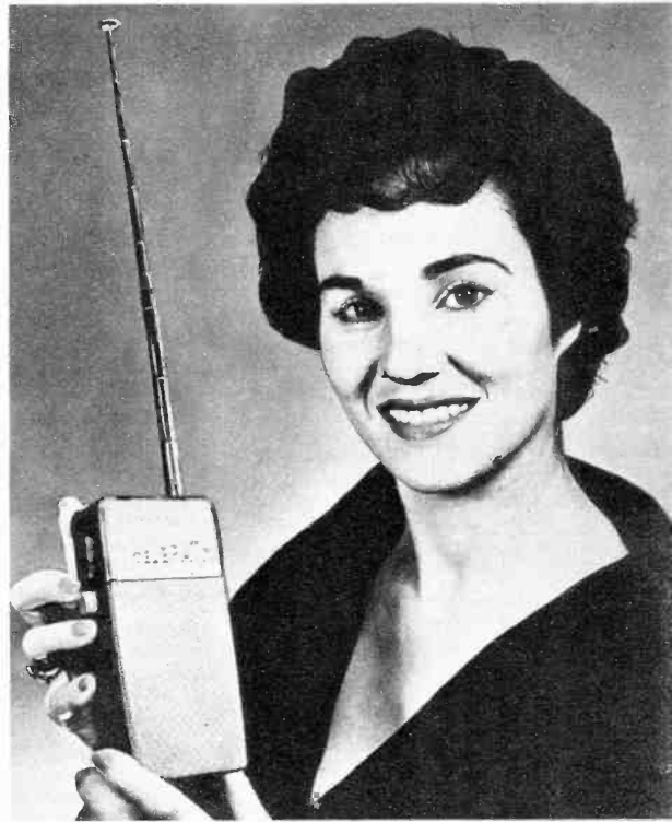
Volume and push-to-talk controls of Lafayette HE-29 are on side of case, leaving front surface free to be placed against mouth for talking. It is powered by just eight standard penlight batteries.
