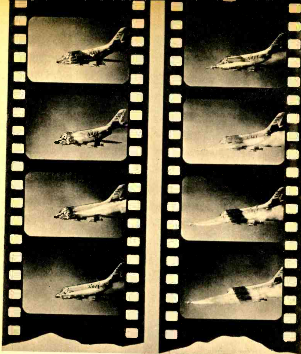
Rapid fire sequence shows Sparrow III, Navy air-to-air missile, being launched from F3H-2 Demon interceptor. Plane carries four missiles which are fired at target automatically when within range. Raytheon Co.
