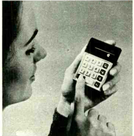
Regen Precision Industries electronic calculator costs $99.95, has eight-digit capacity, works on ordinary batteries, has liquid-crystal display.
