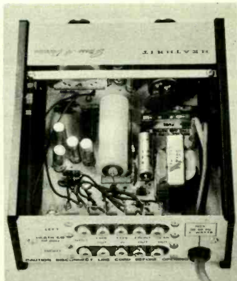
Rear panel of Heathkit is easy to figure out. Although pc board is tighter than Metrotec's, all component locations are clearly marked.
