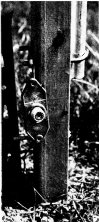
Fig. 1—Diagram at right shows construction details and dimensions. Solder radials to fence post. Photo below is of base of antenna. SO-239 connector is mounted in special holder. Mount it similarly in Bakelite. Connect inner lug to antenna and connect the shell to the fence post.
