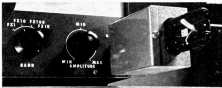
Fig. 1—Generator is built in a 3 1/4 x 2 1/4 x 1 1/8-in. Minibox. On back are chassis-mount banana plugs which fit in jacks on sine-wave generator. Square-wave output at front is available at dual five-way binding posts. Unit is powered by input sine-wave.
