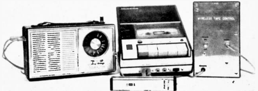
Fig. 1—Complete wireless tape-recording system consists of an FM radio, an FM wireless mike, a reel or cassette recorder and our control box at the right.
