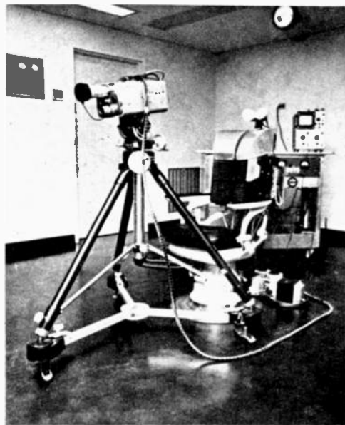
Fig. 2—Tactile TV in lab. Note converted dentist's chair with electromagnetic probes on back.
