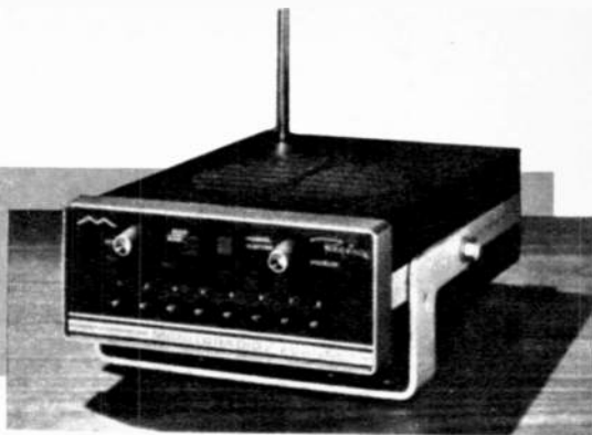
Fig. 5—The receiving robot, Regency's TMR-8. Receiver automatically searches for signals on selected frequencies with eight crystals.
