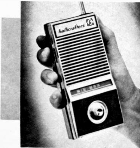
Figs. 2 and 3—Photo at left is of the Hallcrafters Portamon portable VHF receiver. Both low- and high-band models are available with adjustable squelch control. Photo at bottom is the Realistic Patrolman which tunes low and high bands. It's $99.95.
