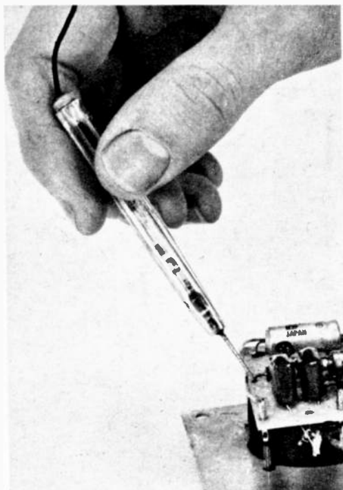
Holder for tester (above) should be clear plastic so you can see glow of gallium-arsenide diode. Note in right photo size of diodes compared to 1/2-watt resistor. Diode D2 is above D1.
