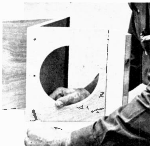
Fig. 3—View of partially assembled cabinet. Diameter of hole in speaker mounting board is 6 \frac{1}{4} in. Attach panels with wood screws and white glue.
