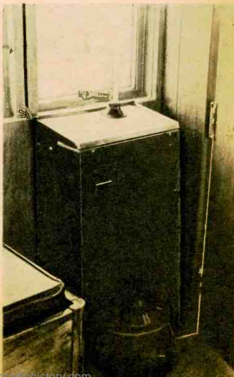
Transmitter-receiver unit for 3-cm radar made by Decca Radar, a British firm. Note small waveguide coming from top. Decca is one of leading suppliers.
