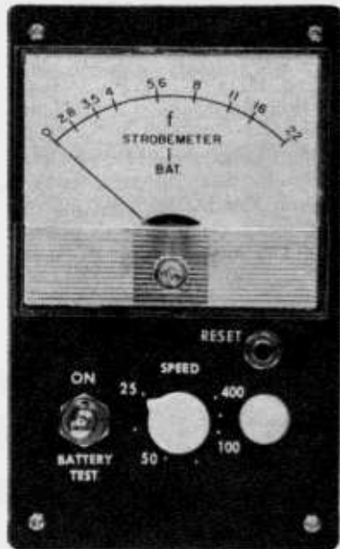
Fig. 6—Finished meter. Switch at left must have center-off position so unit can be turned off completely.
