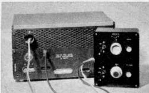
Fig. 5—Rear of modified Hallicrafters S-38E receiver. Connections for R6, S3 are made with tube base (upper left). Other connection is below.
