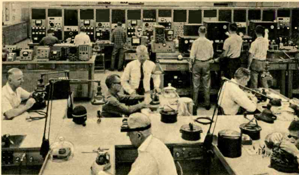
When more than routine maintenance is needed, airborne electronic gear is replaced by standby equipment and the defective unit brought to a facility like this one in TWA's Kansas City, Mo., overhaul base.
