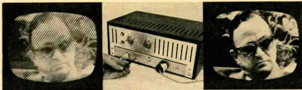
Text explains how to adjust trap on CB (center) to clear hatching on TV caused by CB second harmonic.
