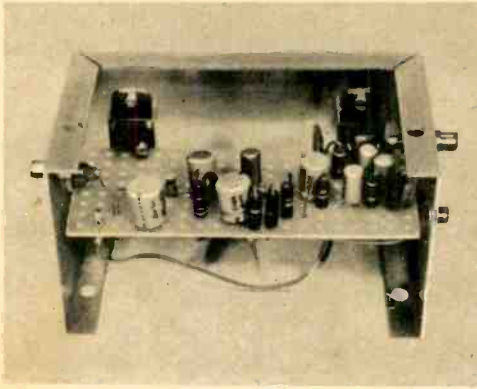
View of top of circuit board. Note how components are mounted on end to save space. Board is supported by lugs on switches and input jacks.
