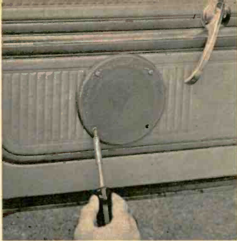
Fig. 4—After you have connected the wires to the speaker, place the grille over the speaker and mount the assembly in door with supplied screws.
