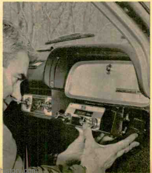
Fig. 7—Polarized connectors assure the correct speaker hookup; fused black wire goes to the ignition switch. Player is installed in mounting bracket.
