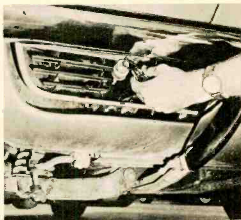
Most systems provide for a hidden defeat switch to allow you to enter car without tripping alarm. Here it is controlled by special lock in grillwork.
