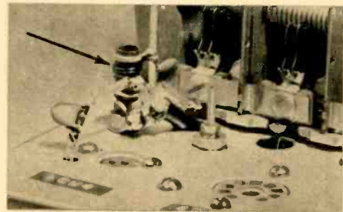
Fig. 4—Closeup of coil L1 (arrow) shows how it's mounted near front section of tuning capacitor. Note coax from J1 coming up through chassis.
