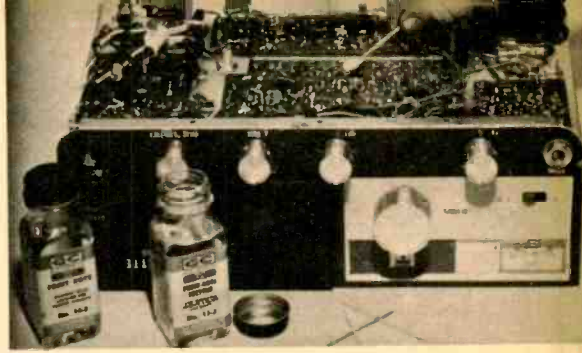
Fig. 3—Protective coating must be removed from PC board with solvent, replaced following repair.
