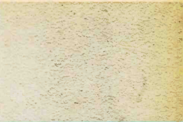
Quality tape displays even distribution of grains under the microscope. Silicon lubrication helps keep these grains from acting as an abrasive.
