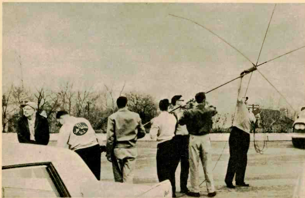
Using the portable groundplane antenna described in this article, the 5-11 Radio Club, Inc., of Pittsburgh, Pa., can be ready with a hefty signal in minutes. Plank base is kept in position by rear left tire of the car in foreground. The folding antenna fits in pipe attached to board like a flagpole in a holder.
