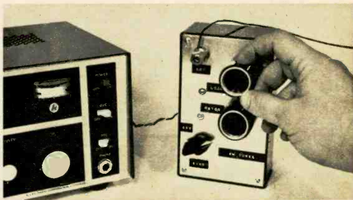
Fig. 1—The antenna tuner should be placed next to the receiver. Variable capacitors and bandswitch are used to make the antenna resonant at the particular frequency you wish to tune. You'll see a difference on the S-meter.
