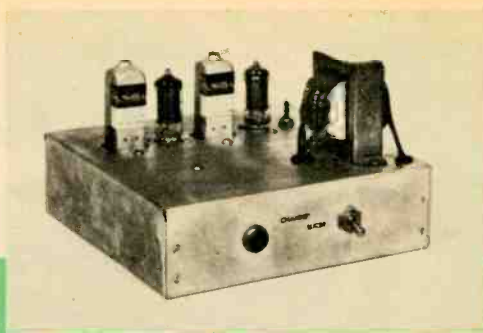
Double-conversion adaptor (here a home-brew) adds IF stage, increases selectivity of some sets.
