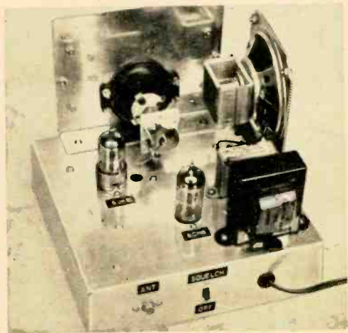
Fig. 5—Plate at front supporting dial assembly is made of scrap aluminum. When mounting the speaker, isolate it from the chassis with grommets.
