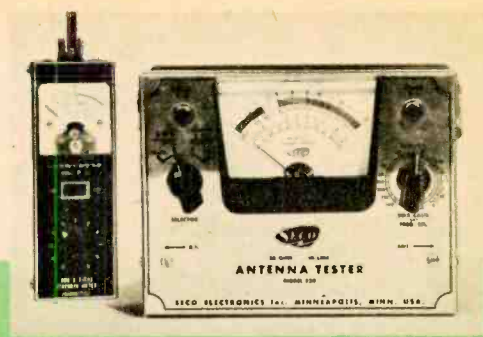
Field-strength meter and combination antenna tester (wattmeter and SWR bridge) check output.
