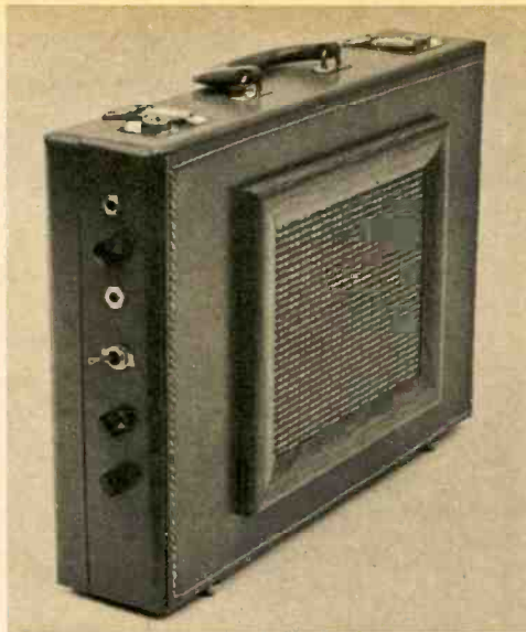
Fig. 4—Top jack is input, control below is volume. Next jack is for tremolo on/off foot switch. Bottom controls are tremolo speed and intensity.
