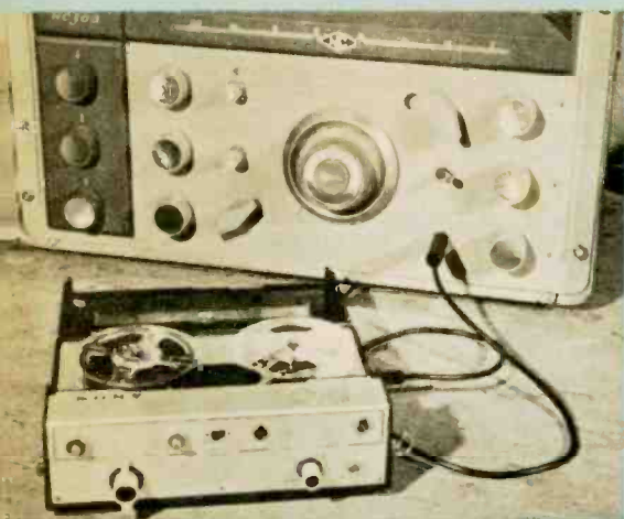
Proper patch cord is about all it takes to add a tape recorder to most any ham shack. Fone jack on receiver feeds tuner input on recorder.
