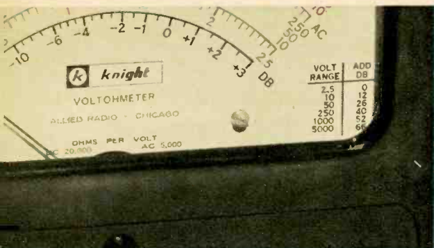
Large, easy-to-read meter scale is significant feature in the cap of any VOM. Db/volts chart (lower right in photo) comes in handy for making audio measurements.
