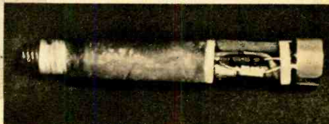
The Basalog transmitter, designed to be worn internally, responds to slight temperature changes by shifting frequency. Signal from transmitter element (below) is picked up to graph temperature as aid to would-be mother.
