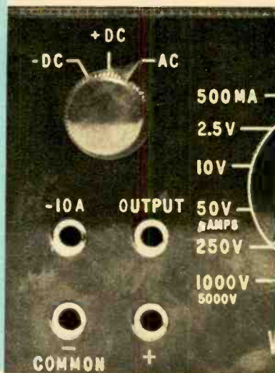
DC reversal switch (at upper left in photo) provides means to reverse the test-lead polarity without interchanging the leads.
