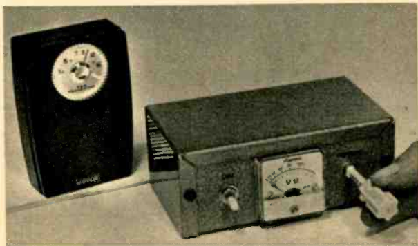
Pager is tuned to an unoccupied spot on the broadcast band by adjusting a front-panel-mounted coil. Radio becomes quiet when Pager is on frequency.
