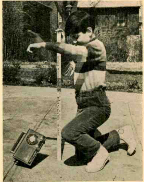
Combination zinc and plastic case ably protects circuitry from bangs and jars most every portable is heir to. Heavy components are shock mounted.
