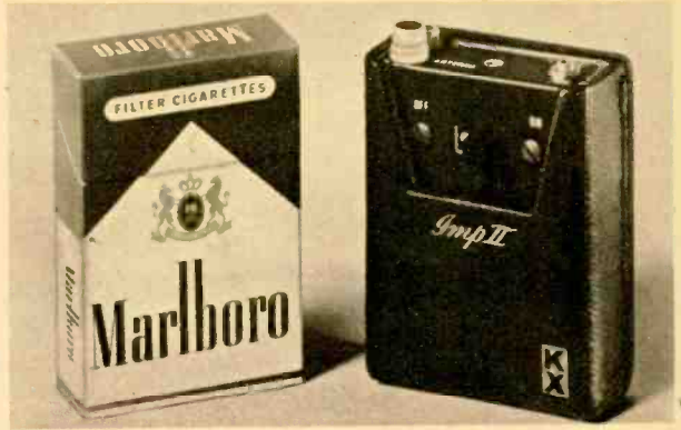
Roughly the size of a cigarette pack, Kinematix IMP II is typical of popular-price FM wireless mikes. Unit covers 30-20,000 cps audio range.
