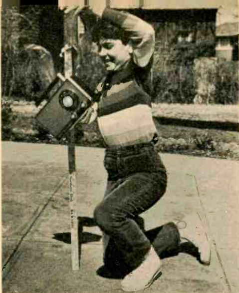
Shock test entailed repeatedly dropping the radio onto concrete from 3-ft. height. Set didn't mind the rough treatment a bit and kept right on playing.
