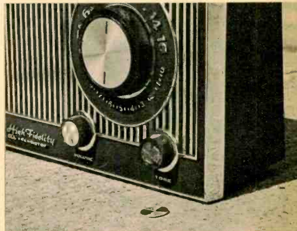
Sole damage produced by stringent shock test was a few small dents in chrome trim and dropping out of decorative metal inset in tone-control knob.
