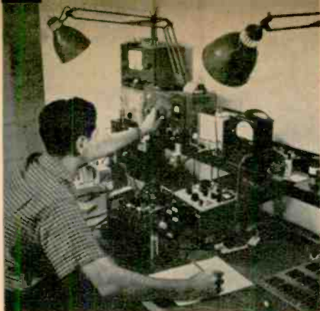
Aging completed, units are aligned with crystal-controlled frequency standard specifically designed for CB rigs.
