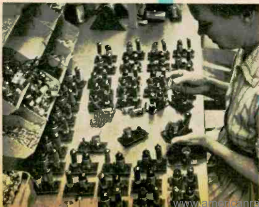
With components mounted in place, board is coated with flux, dipped in molten solder.
