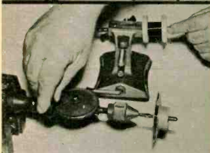
Remove flange from 8mm film reel, slip on cardboard disc 3/16 inch from other flange, then wind 1,000 turns.
