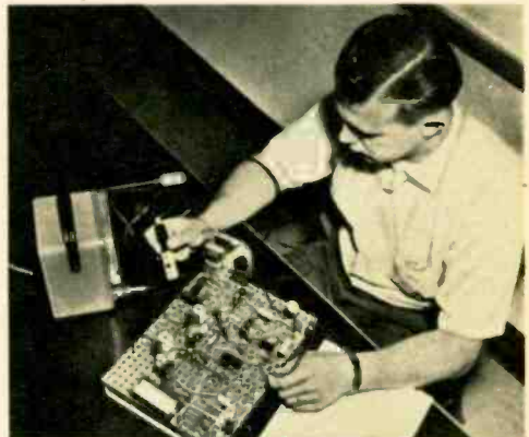
Circuit board from ICS is ideal for experiments. Parts are clipped rather than soldered in place.
