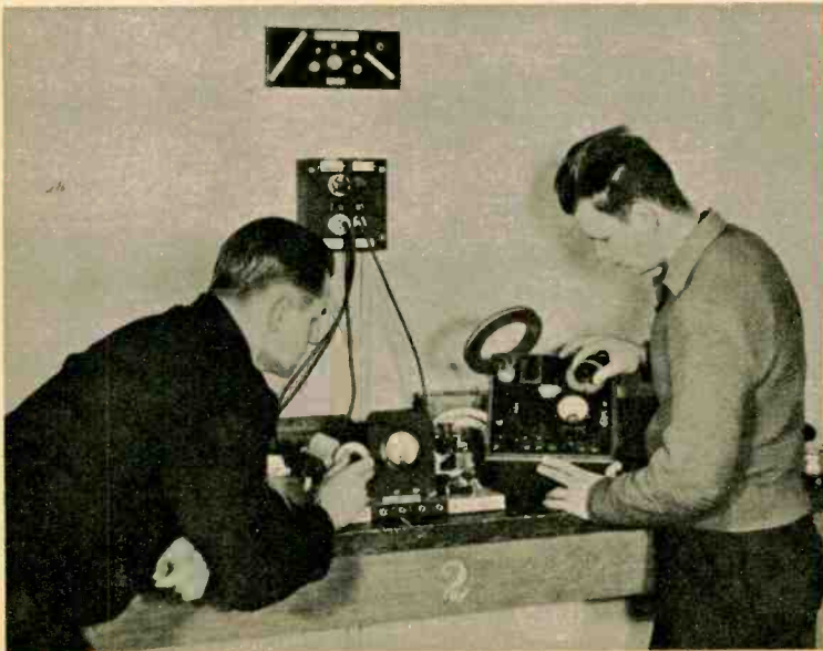
Spark gaps and CW ruled the roost decades ago, and radio inspectors relied on an instrument called a decremeter to check up on those sparks. Reason was that a signal which decayed too rapidly when the key was open likely would cause severe interference. Our photo shows students testing out a Kolster decremeter in the laboratory of a Seattle, Wash. radio school back in the early 1920's.
